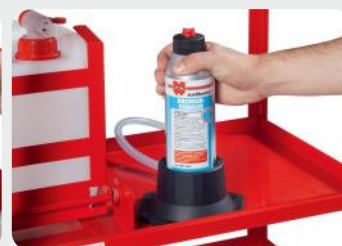
3. Place the bottle on compressed-air filling station.
